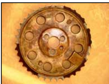
A broken nylon cam gear.
