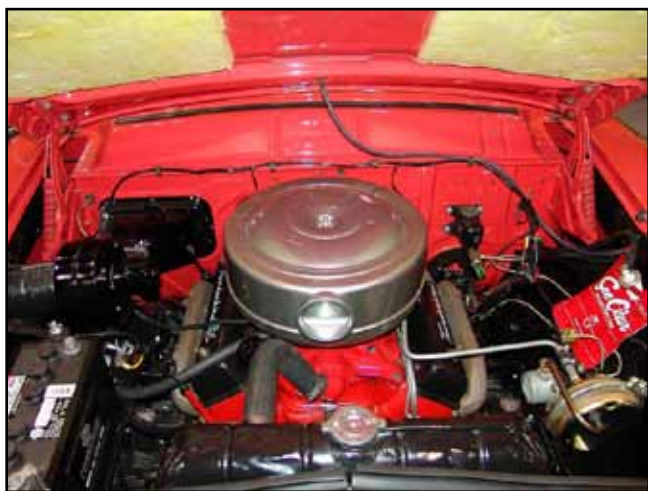
A good old Y-block Ford engine with a “teapot” carburetor!
