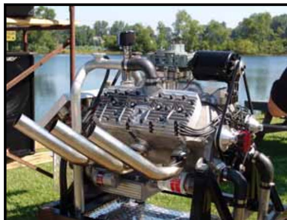
The long awaited aluminum flathead V8 ready to run.
