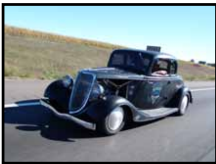
The "mule" with the aluminum flathead V8 in it.
