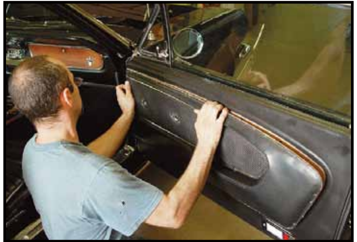
The interior is carefully disassembled.
