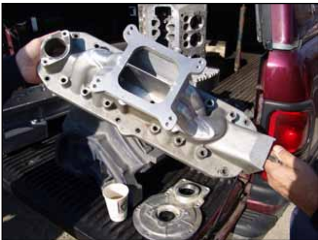
Intake manifold showing enormous plenum.
