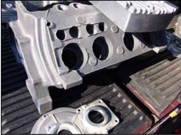
Close-up detail of the raw block casting.
